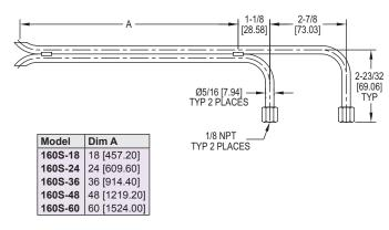
The Series 160S "S" Type Stainless Steel Pitot Tubes are designed specifically for flow measurement of dirty, particulate laden air or gas streams typical in smoke stack and other environmental testing. Total and static pressure tubes are precisely aligned and welded together every 6 inches for maximum accuracy, strength, and long term durability. Permanent mount (PM) models include a 1" welded stainless steel sleeve and adjustable compression fitting with 1" MNPT mounting threads.
